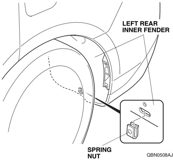
12. Loosely install the left rear splash guard to the left bracket and left rear inner fender with one 5 x 20 mm self-tapping screw provided and two self-tapping screws removed in step 7.
