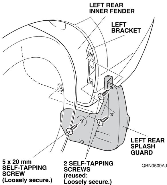
13. Loosely secure the left rear splash guard to the rear bumper with one additional 5 x 20 mm self-tapping screw provided.
