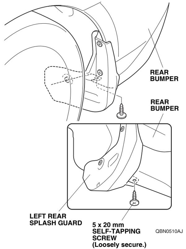
14. While holding the left rear splash guard against the rear bumper, tighten the four self-tapping screws in the order shown.
